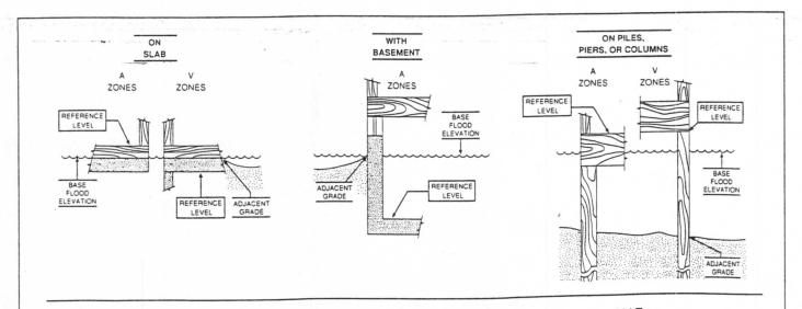
The diagrams above illustrate the points at which the elevations should be measured in A Zònes and V Zones.
