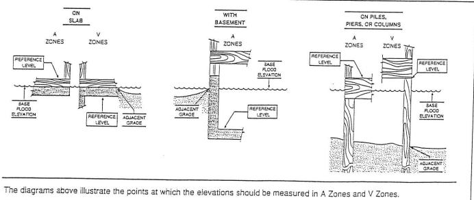
Elevations for all A Zones should be measured at the top of the reference level floor.
